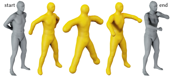
Fig. 3. Simply penalizing the total repulsive potential over a time-varying trajectory yields undesirable deformation: between the fixed start/end configurations, the surface “explodes” away from itself to reduce potential.
