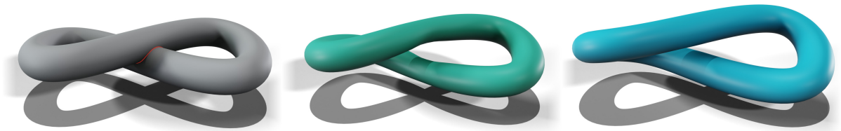
Figure 6.12: Fixing intersections in a given mesh (gray, intersections in red) by decreasing the sub-repulsive tangent-point energy using a trust-region method (green) leads to undesirable deformations of the shape. In contrast, decreasing the combination elastic and sub-repulsive tangent-point energy (blue) allows preserving the overall shape while removing the self-intersection.
