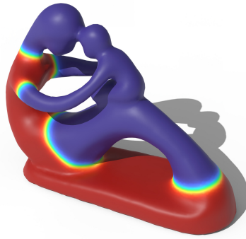
Figure 8.8: Distortion minimizing segmentation of the ‘fertility’ model (courtesy of the AIM@SHAPE project). Interface width is given by \varepsilon = 0.02 and the distortion weight by \omega = 0.1 . For this example, minimizing (8.20) yields segment boundaries following paths with negative Gauß curvature.
